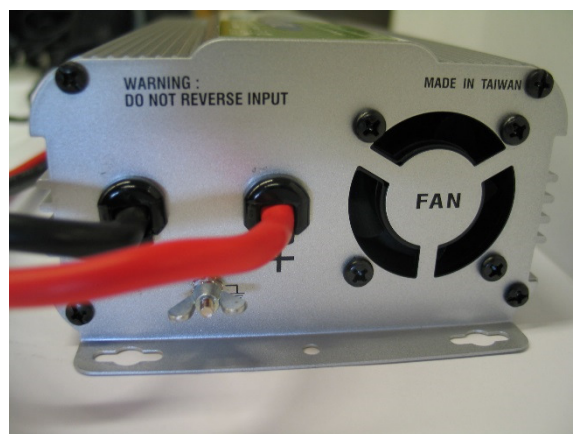
Picture 6: Backside DC cable input PE connector
