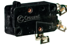
Customised version for nuclear application. Has radiation-resistant housing, 180 °C max operating temperature, W5 screw terminals and magnetic blowout for highly inductive circuit switching at 250 V \overline{\text{=}}
